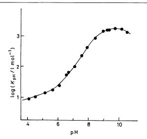
Variation of the equilibrium constant for the formation of the Schiff's base between PLP and n-hexylamine as a function of the pH, at 15 °C. • Experimental values calculated from  $k_1/k_2$ . The line is calculated from equation 6 and the parameters are given in Table 5
